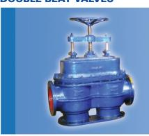
Details of Application: Juice Heaters Size Range (dia): 100 mm to 300 mm Material of Construction: Cast Iron / MS Fabricated / SS Fabricated Internals: Stainless Steel / Rubber
